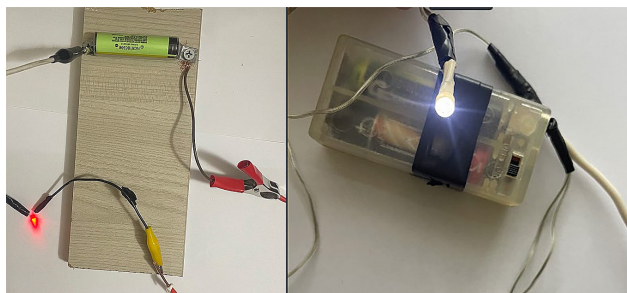
Figure 4. Devices for testing the electrical conductivity of substances, made by the pupils of the experimental class themselves
